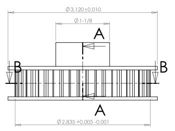
NOTE: CORED PULLEYS HAVE 1/16" THICK RIBS, REINFORCEMENT
